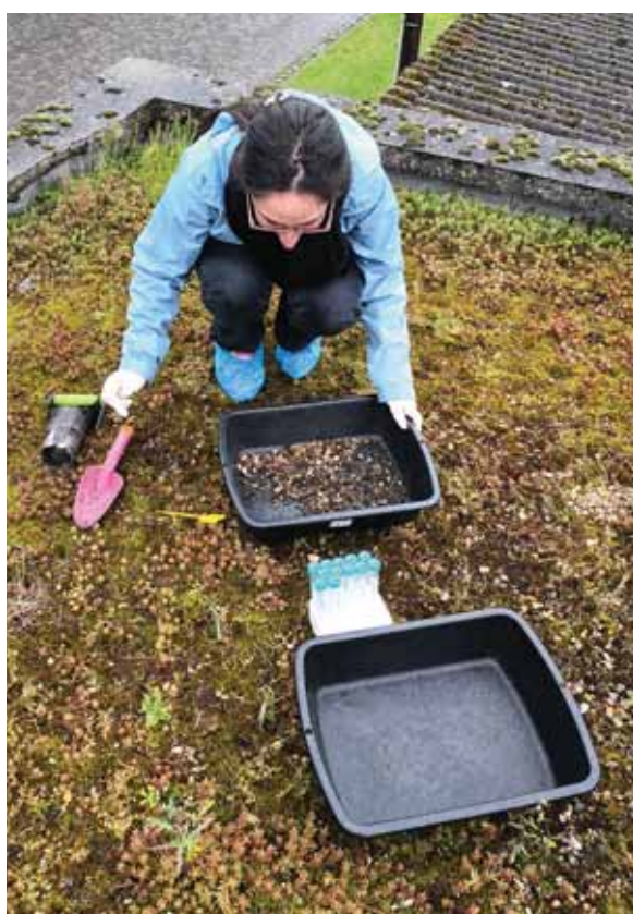
Pooling the 10 soil samples on the roof of the technical building of the Conseil Départemental of the Val-de-Marne. © Marc Barra | ARB îdF
